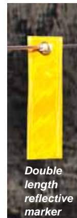
CAB Extra High Visibility Lifeline is easily seen from any direction in escapeways. Lifeline markers hang vertically so they can be seen for long distances up and down escapeways. Markers are flexible so miners' hands can slide easily over them.
