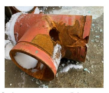
Attached is a picture of two of our failed backfill "T"s. These components generally last two weeks to a month. We installed a Polytec "T" in one of our high wear areas last year and it is still in service. We are in the process of replacing all current "T"s in service with Polytec "T"s. We expect to see improvements in system reliability not to mention safety considerations.
